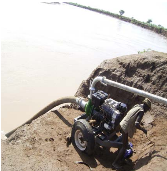
3-cylinder engine water pump, pumping water from Omo Rive to the irrigation land.
